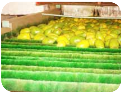
Figure 5. Cactus fruit cleaning machine in Mexico
