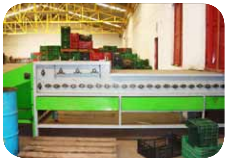
Figure 5. Cactus fruit cleaning machine in Mexico
